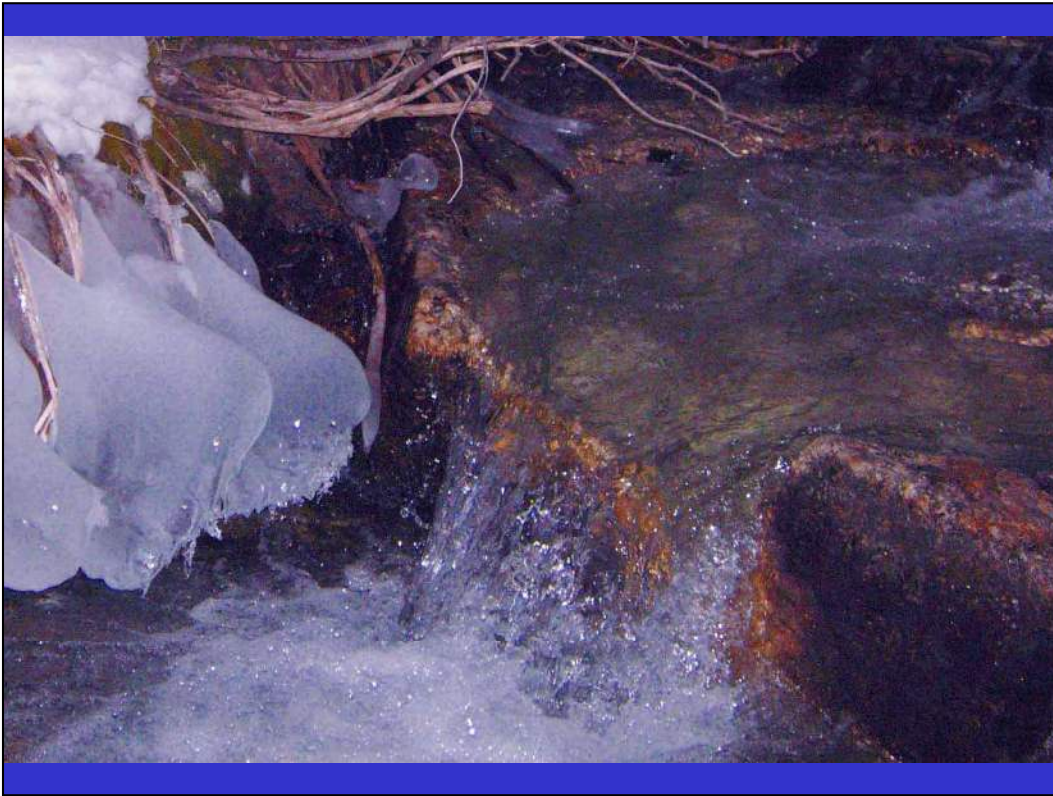
Photo of arastra from downstream. The downstream lip of the arastra has broken off and acts like a spillway.
