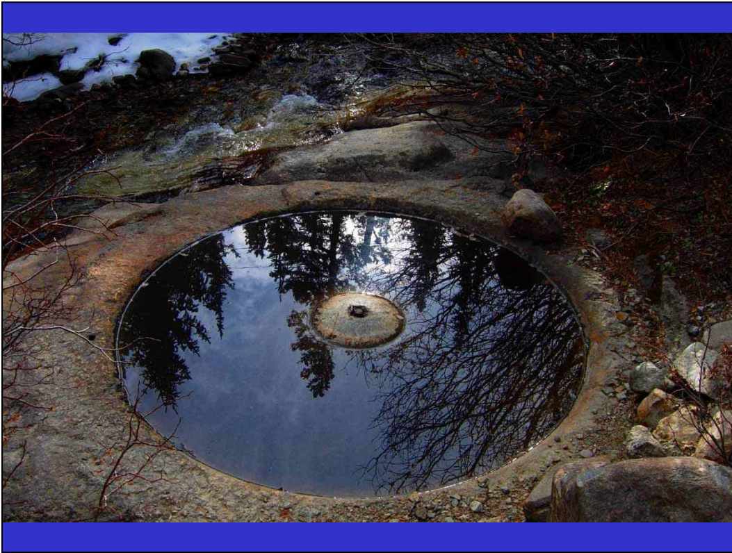
Photo of same arastra. The central high point shows the remains of a steel post that the yoke and heavy stones were attached.
