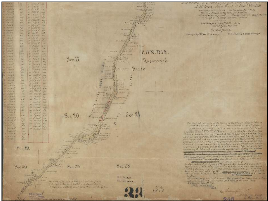
An early gulch placer claim example in Montana that is approx. four miles long. The great majority of the corners are trees or stakes with mound and pit.
