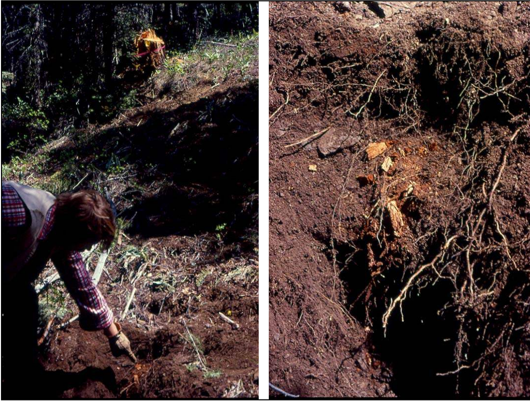
Freshly cut bearing tree for the remains of the sub-surface mineral survey corner post.
