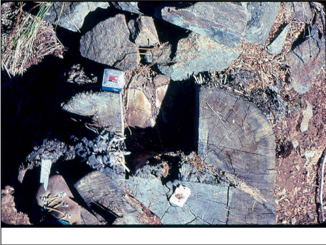
A vertical view of the overgrowth seam and the flat face on the suspected (accepted) pine tree stump for Corner 3, MS 956A.
