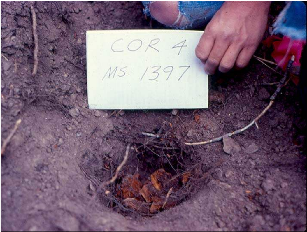
Remains of a sub-surface mineral survey corner post found by intersecting a distance-distance tie from the nearest found mineral survey corners.
