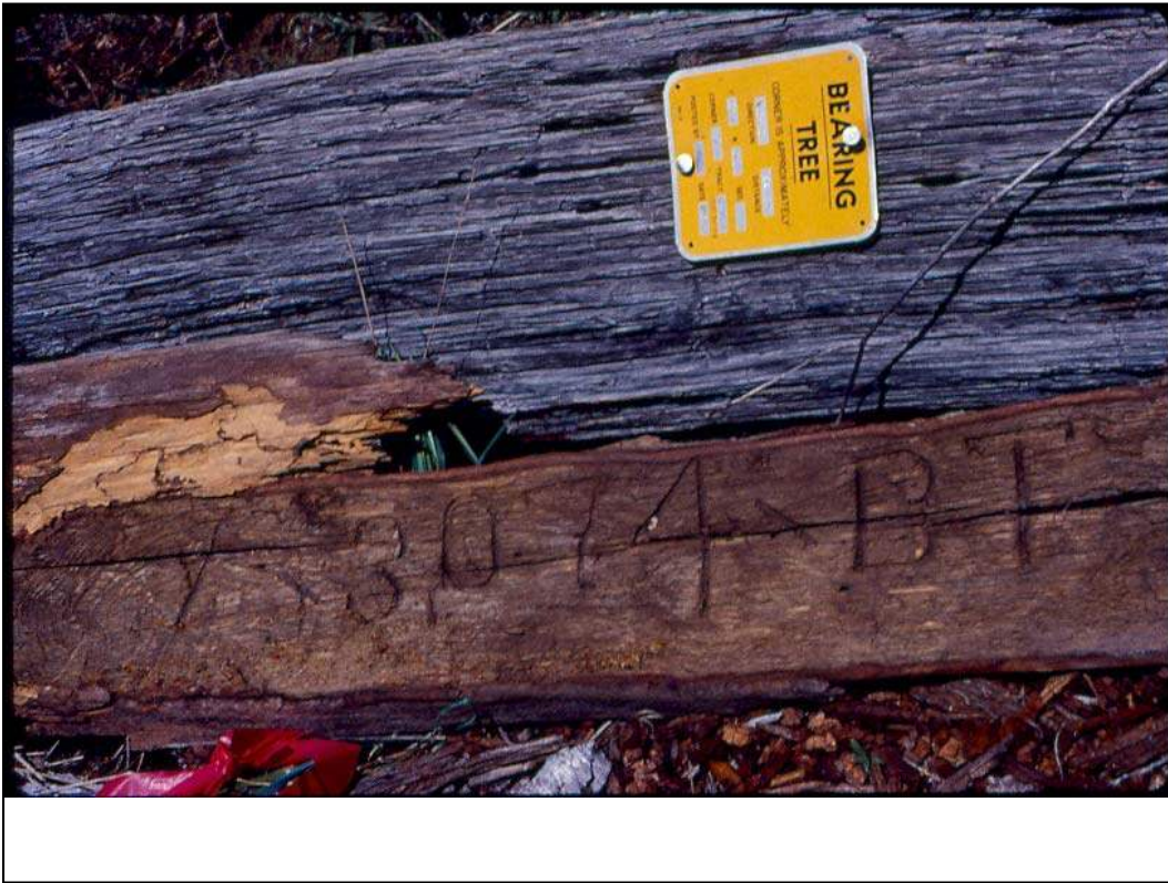
Forest Service Bearing Tree sign and one of the bearing trees for Corner 5, MS 3074, Ureka Lode.
