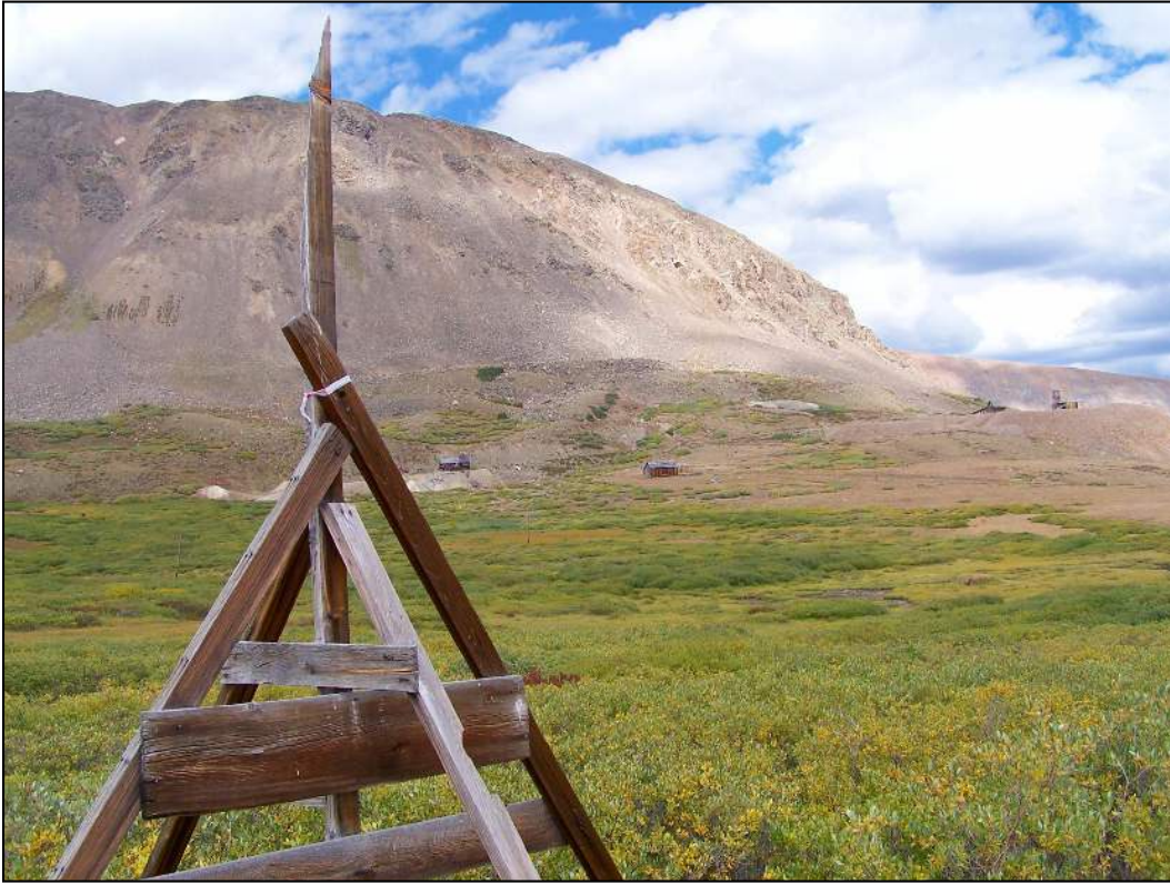
Photograph of a permanent backsight erected at the SW Cor. Sec. 7, T. 9 S., R. 78 W., 6 th P.M. looking to the northeast at the mining claims described above with London Mountain in the background.
