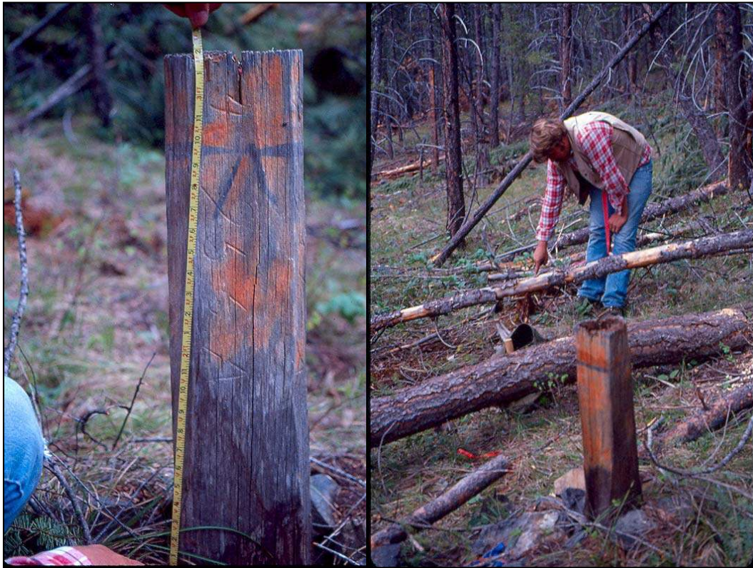
Original scribed wood post for Corner No. 4 (SW corner) of MS 956A, on left, and surveyor pointing to the rotted remains of a bearing tree witnessing said Corner No. 4.
