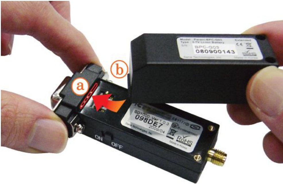
Figure 2-6 Attach the battery pack
