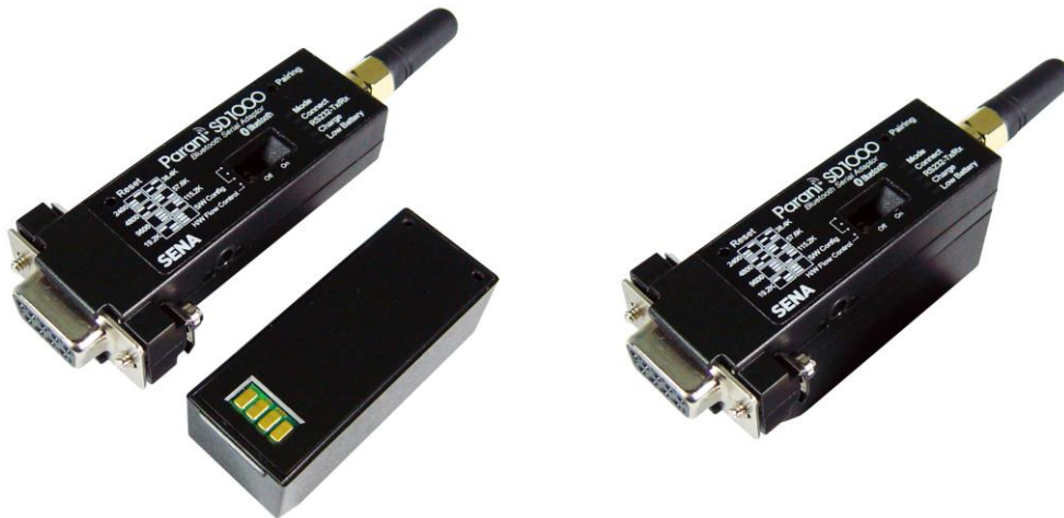
Figure 2-4 Attaching Battery Pack to Parani-SD1000
