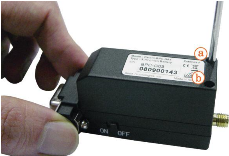
Figure 2-7 Fasten the battery pack
