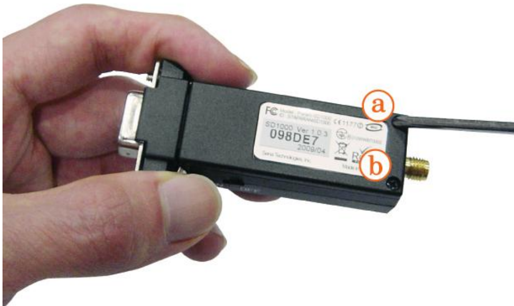
Figure 2-5 Remove Parani-SD1000 bottom cover
