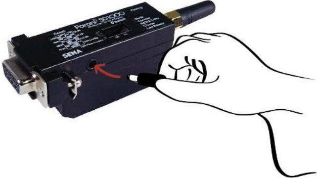
Figure 2-2 Connecting Power to Parani-SD1000
