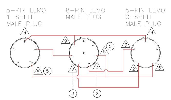
LOOKING INTO PLUGS. NOTE THAT THE PLASTIC BLOCK (NOT SHOWN) APPEARS TO CONTAIN DIODE(S) FOR REVERSE POLARITY PROTECTION.
