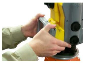
Figure 3.2 Attaching the ACU
