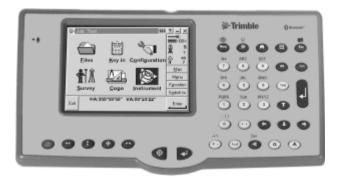
Figure 3.1 The ACU controller – front view
