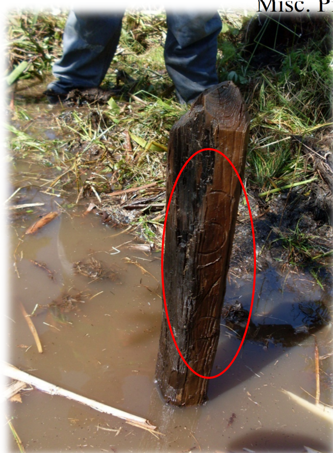
Wood post, set in early 1900's by a surveyor working for the International Harvester Company. Recovered by BLM in 2008. Located in an old Tamarac swamp on WEIR. Upper left picture has some of the scribing visible. Upper right picture is of entire post. Lower picture is of the post stood up and the crew consisting of Tom Uran (left front), Doug Uran (left back), and Brett Tibbetts (right).
