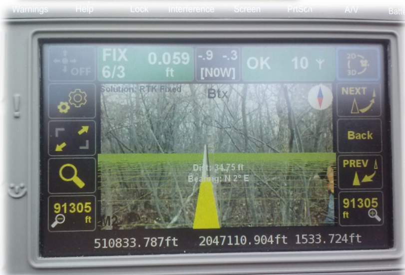
Screen of a modern GNSS rover. It uses a camera on the front to show the distance and direction to a point as a heads up display.
