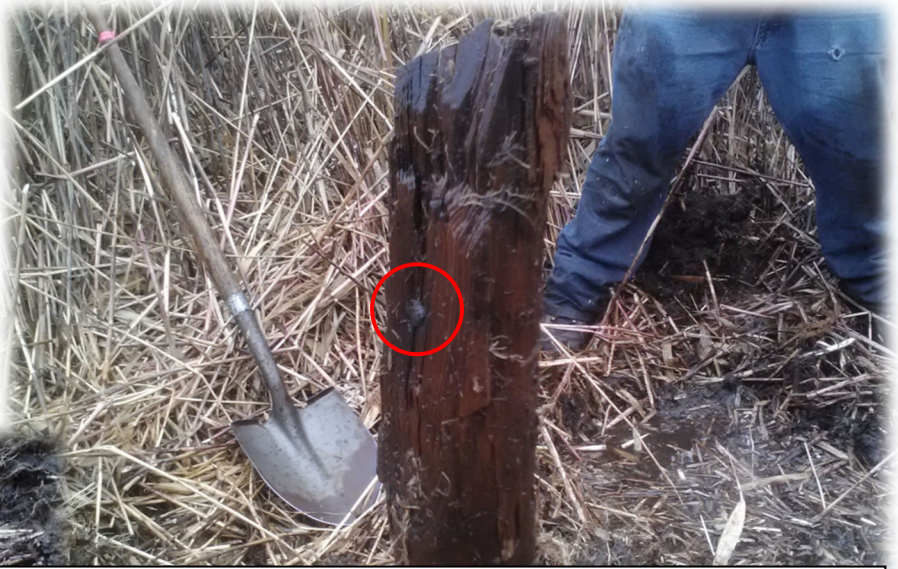
Wood post, originally set in 1870, recovered by county surveyor in 1899 for highway survey, again recovered by BLM in 2012. \frac{1}{4} cor. of secs 21 and 22 of T. 135 N., R. 41 W., 5th P.M., Minn. The post has a brass tack (red circle) assumed to have been placed by the county surveyor and the other wood posts are most likely witness stakes or flag posts set in the late 1800's. Lower left picture is of the original bearing tree, the blaze is visible as a flat pitched up area (yellow circle).
