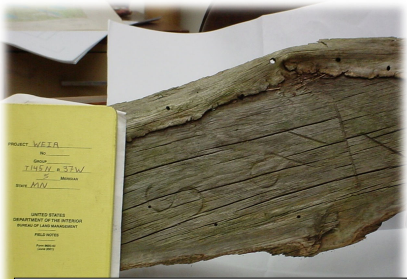
NW 1/16 of sec. 26, T. 145 N., R. 37 W., 5th P.M., Minn. This corner was established and set in 1890 during a resurvey of a township to subdivide the sections into 40 acre tracts for the purpose of issuing Indian Allotments on WEIR. The section subdivision was not done in the normal manner as they were run east and west through the section on random and true lines (3-mile method). The pictures are of the bearing tree marked in 1891 and recovered by the BLM in 2007. The left picture is the actual blaze with scribing visible, which came from the area of the stump in the right picture circled with a large yellow oval. The small yellow oval is a blaze that would have been marked BT.
