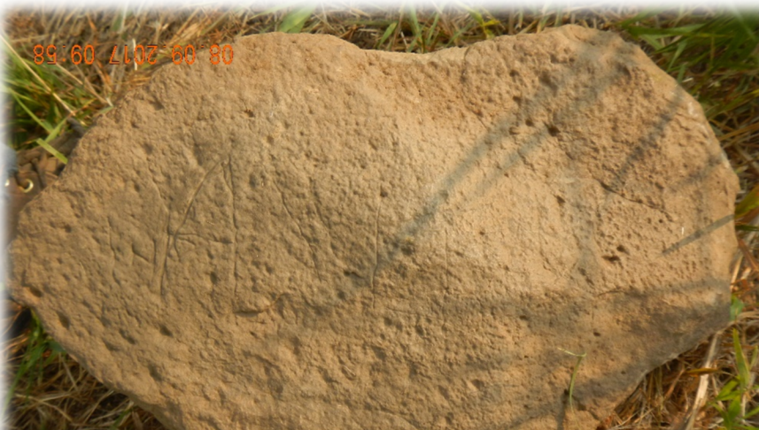
This stone was set in 1892 for a corner (sec. subdivision cor.-1/1024th-every 2½ chains) of Indian Allotment No. 56 on the Nez Perce Indian Reservation (NPIR). It was set by the same GLO contract surveyor that surveyed the township to the extent necessary for surveying the allotments per the Indian Agent's instructions. No record of the allotment surveys has been found to this day, so searching for corner evidence is difficult to say the least. The marks appear to be an attempt at roman numerals for the allotment number. The interpretation is IND (Indian) A (allotment) XLI (actually 41 but should be LVI). Again, it appears the marks were scratched in instead of chiseled. This particular surveyor had crews consisting of inexperienced Tribal members hence the odd marks and mistakes. Recovered by BLM in 2018.
