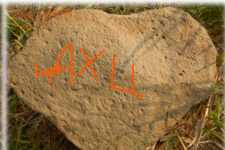
This stone was set in 1892 for a corner (sec. subdivision cor.-1/1024th-every 2½ chains) of Indian Allotment No. 56 on the Nez Perce Indian Reservation (NPIR). It was set by the same GLO contract surveyor that surveyed the township to the extent necessary for surveying the allotments per the Indian Agent's instructions. No record of the allotment surveys has been found to this day, so searching for corner evidence is difficult to say the least. The marks appear to be an attempt at roman numerals for the allotment number. The interpretation is IND (Indian) A (allotment) XLI (actually 41 but should be LVI). Again, it appears the marks were scratched in instead of chiseled. This particular surveyor had crews consisting of inexperienced Tribal members hence the odd marks and mistakes. Recovered by BLM in 2018.
