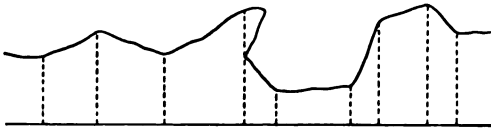
FIG. 48.—Offsets to Irregular Boundary.
