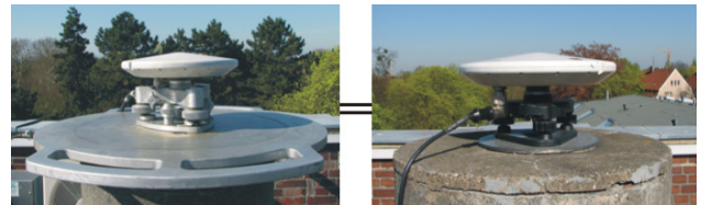
Figure 21: Pillars with rover antennas (setup B2, B3).
