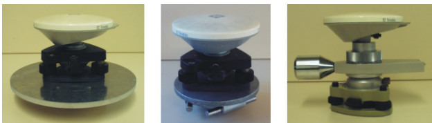
Figure 5: Antenna test candidate TRM39105.00 mounted over the metal plate (left), the tripod head (middle) and the special adaption for fixing a leveling rod (right).
