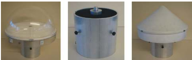
Figure 6: Antenna test candidates TRM41249.00_TZGD (left) and LEIAT503_LEIC (right) mounted on a metal cylinder (middle).
