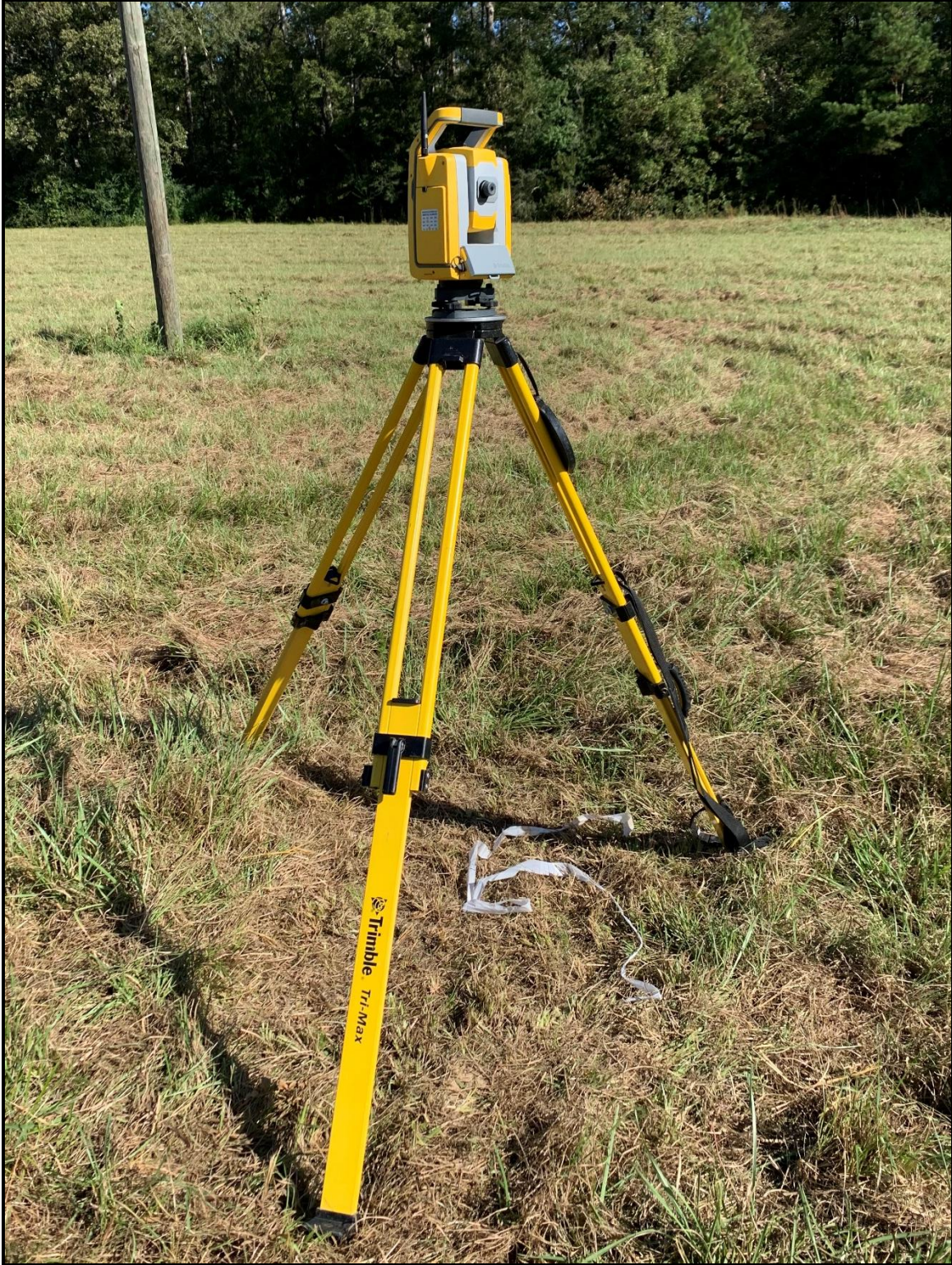
Figure 5 – Trimble S5 5” robotic total station setup on PT002.
