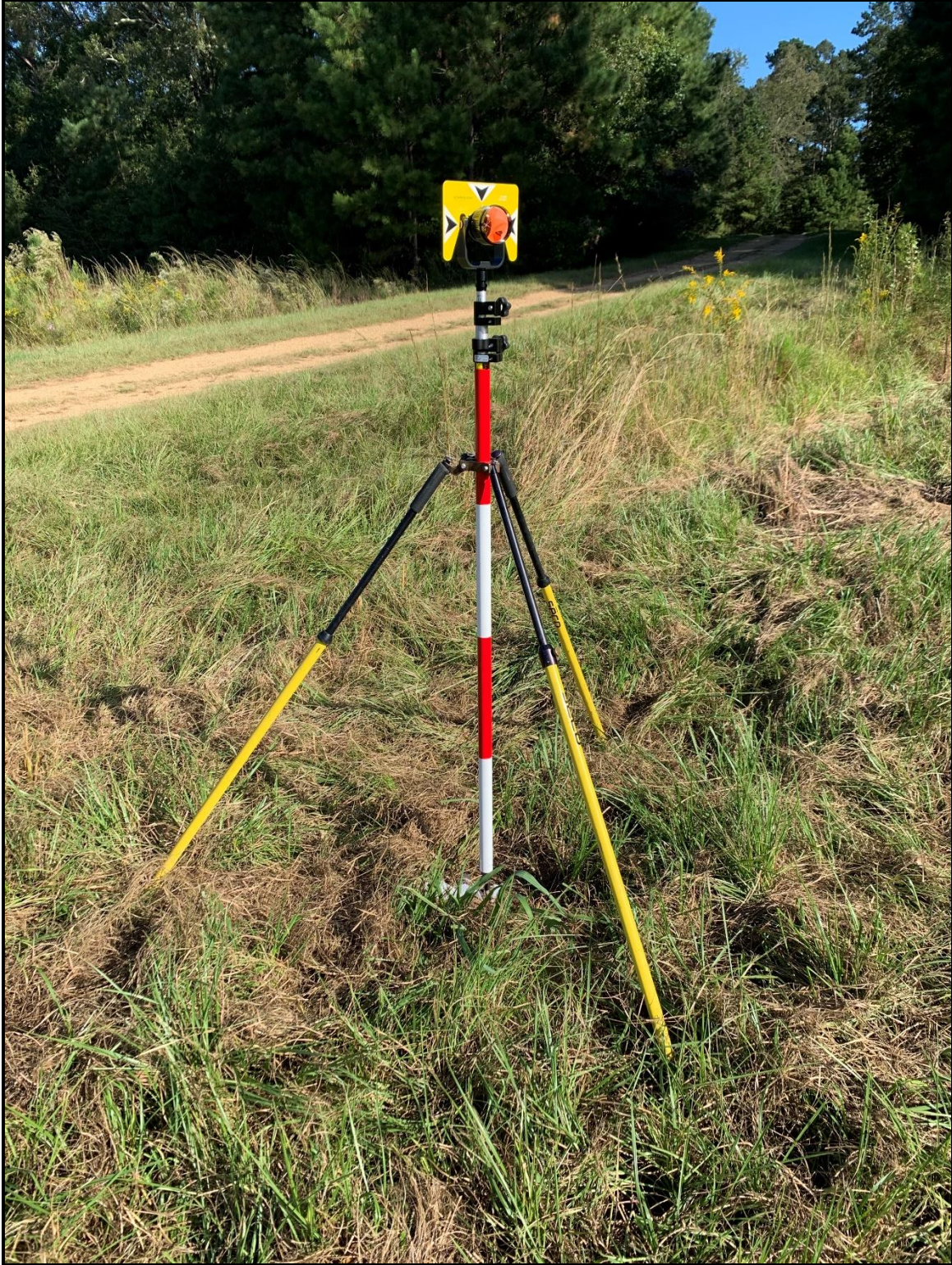
Figure 6 – Backsight prism setup on PT003.
