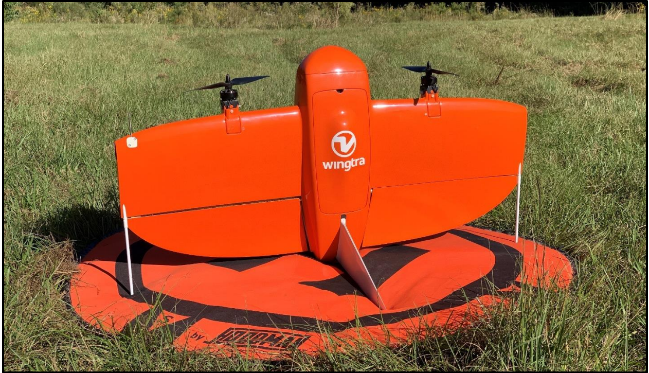
Figure 9 – WingtraOne UAS, equipped with Sony RX1RII camera and PPK system.
