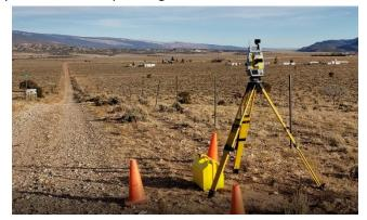
Once setup and locked on the prism, the Pixel 4a was disconnected from the robot both were transported to approximately 2,500-foot distance while maintaining lock.
