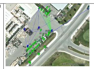
Two step method: Combine GNSS and total station by first computing points with GPS, constraining to these coordinates and then adding conventional data.
